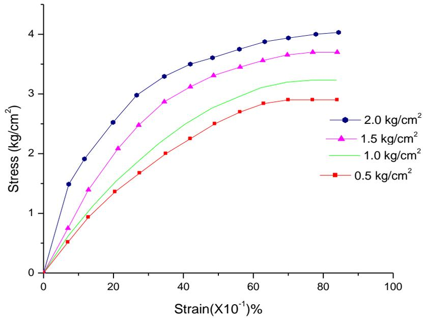
**Figure 4:** (c) Stress-Strain Curve of Bentonite + Acetic Acid
