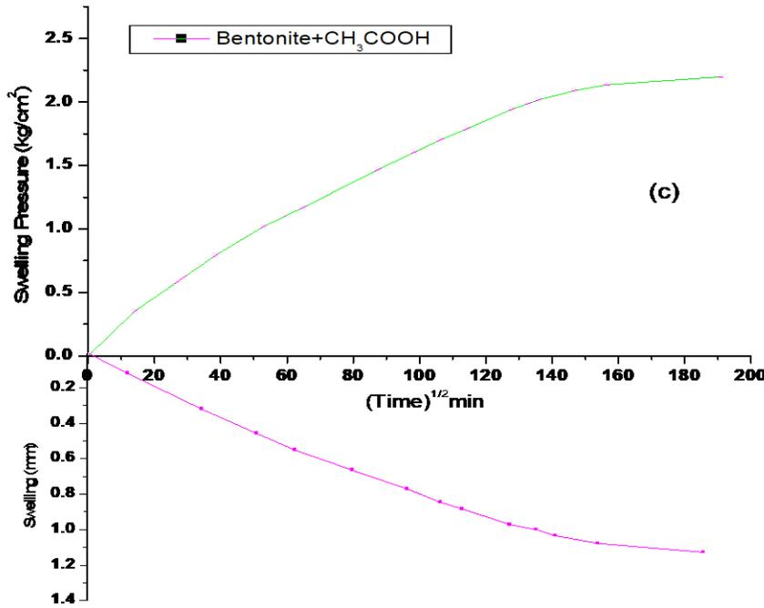
**Figure 5:** Influence of Chemicals On Swelling Pressure and Swelling of Bentonite soil
