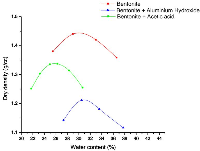
Figure 3: Influence of Chemicals on Compaction of Bentonite
