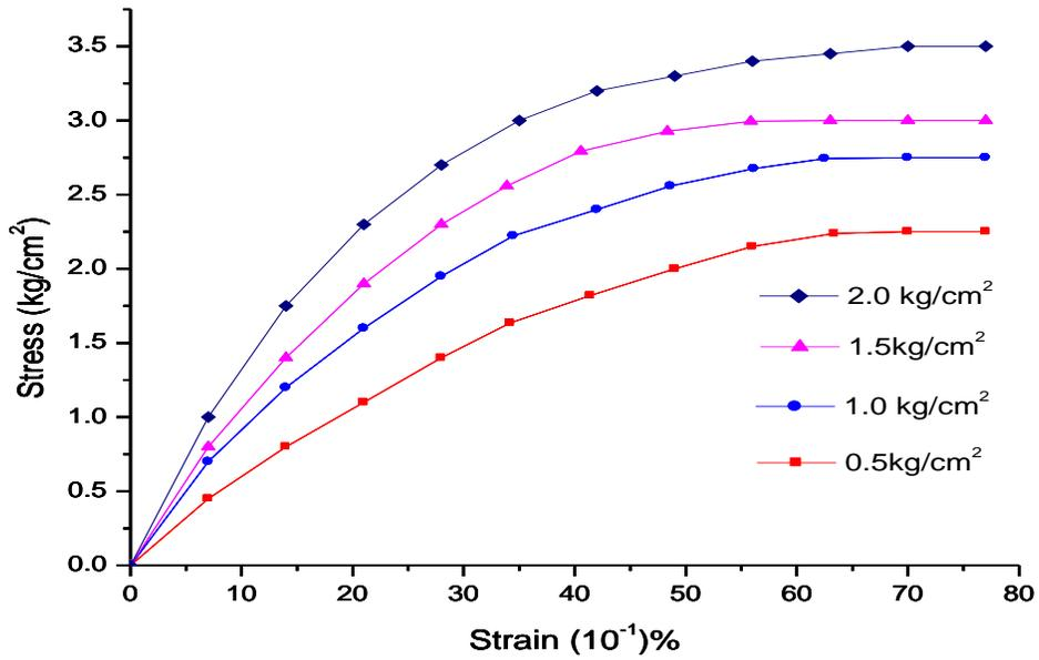
Figure 4: (b) Stress- Strain Curve of Bentonite + Aluminium Hydroxide
