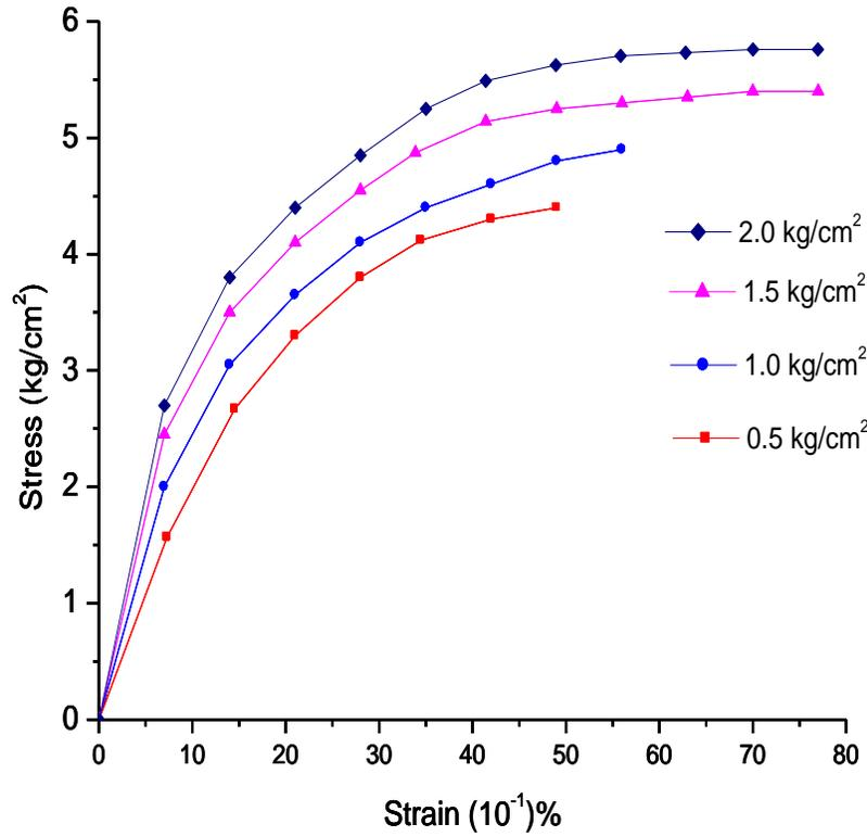
Figure 4: (a) Stress-Strain Curve of Bentonite alone
